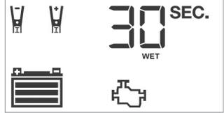
The Pump Engine Icon flashes. The Digital Display shows the countdown to indicate the unit is in Engine Start Mode. The bars on the Battery Icon will change from empty to solid (bottom to top) repeatedly. The Clamp Icons, the Battery Type Indicator and the Battery Icon will light solid.
