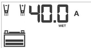
The Digital Display shows the output current that is charging the battery. The Clamp Icons and the Battery Type Indicator light solid and the bars on the Battery Icon will change from empty to solid (bottom to top) to indicate the unit is in Charging Mode.
