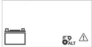
The Fault Icon will flash. The Alternator Icon, "ALT" and the (empty) Battery Status Icon will light solid.
