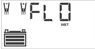
The Digital Display shows "FLO" indicating that the unit is in Float Charge Mode. The Clamp Icons, the Battery Icon (with three bars), and the Battery Type Indicator will light solid.
