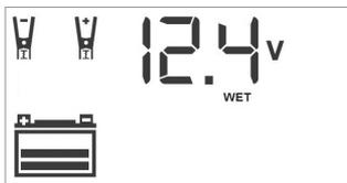
The Digital Display shows the voltage of the connected battery. The bars on the Battery Icon represent the charge level of the connected battery. The Clamp Icons, Battery Icon and the Battery Type Indicator light solid.
