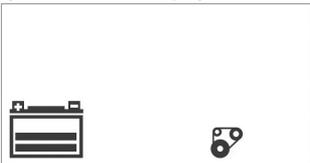
The Alternator Icon will flash and the Battery icon with two bars will light solid.
