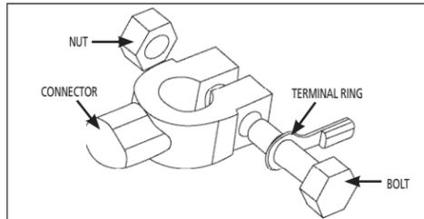
1. Remove the nuts from the bolts of the battery post's connectors.
