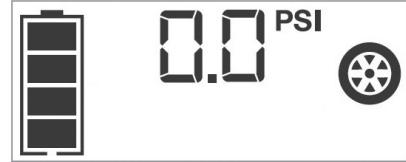
The Compressor Icon will light and the Digital Display will alternately show the flashing pre-set psi value (that was last set by the Compressor Pressure Control Buttons) and the current pressure of the item being inflated (which will light solid).
