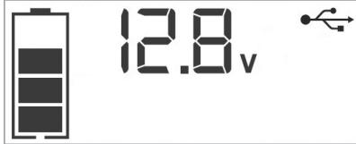
The Battery Status Icon and Battery Voltage Indicator will light solid, as well as the USB Icon, indicating the USB Ports are ready to use.
